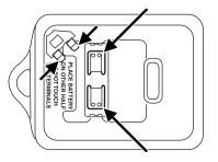
orientation of the battery. Press the battery down to ensure that the battery is fully seated in the battery housing cavity.
